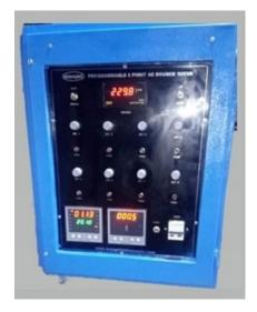
This source is equipped for life testing (Ageing) of any type of electrical appliances / lights / fans by inserting different voltages for different time intervals which are pre-settable in multi channels. It is available in different models from 2 KVA to 100 KVA in single and 3-phase models with output voltage 90 V – 325 V AC. Output current can be monitored and limited for safety purposes also.
