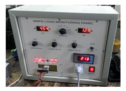
Multi output SMPS supplies used in computers and other applications are tested on this equipment. This is basically an electronic load bank and is used to measure the capacity of any type of DC supplies with independent settings of all six /desired channels. It's a smart testing of your power pack with electronic load hanging over it. The load is in continuous variable type. It is portable, low-cost, general-purpose, easy to use and versatile
