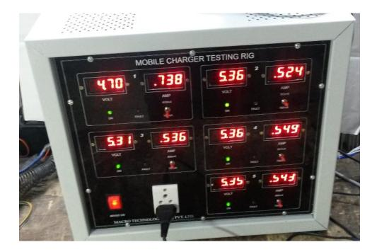
This is custom build equipment made for particular PCB / panel to test on desired electronic load with pass fail indications to test components and board before fixing in housing.
