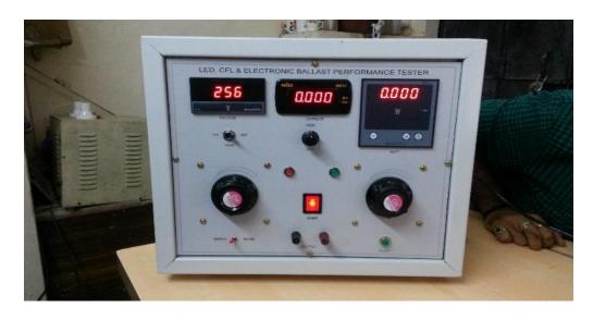
This instrument is used for LED Lights and other electrical products which tested at the time of production, QC. It provides all type of tests by clicking one push / foot switch like series test, normal voltage parameters test, low voltage test, high voltage test for jerk testing of such products.
