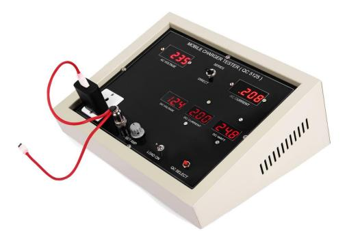
Mobile charger tester with three protocol software to shift 5-9and 12 volt automatically is used to test the circuit of mobile charger for production with variable electronic load up to 5Amp i.e. 60 watt to ensure the quality of product. It is equipped with variable electronic load to set current at desired value with series fail indication, input / output, voltage / current and ok / fail indication.
