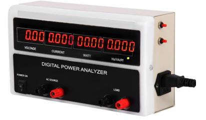
Digital power analyser is compact portable easy to use for finding all six parameters to approve and compare the quality of any type of electrical appliances or device with digital display of voltage, current, apparent power, power factor, wattage as well as frequency of given ac source and load
