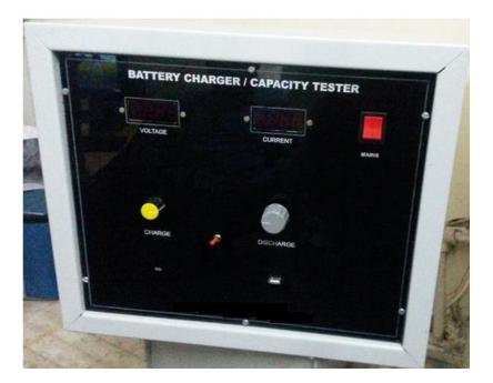
This equipment is used to test the quality of battery by charging/discharging battery/power bank at desired current and voltage.
