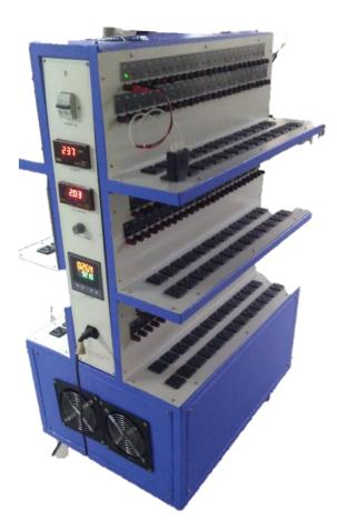
This is multipoint variable type load panel for adopter/chargers and SMPS supplies it tests lot wise bulk items at full load for desired time and sort out the fail or undervalued pieces with any type of manufacturing defects before to improve quality and avoid field failure
