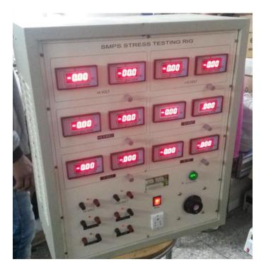
SMPS supplies used in computers can be tested on this RIG. This is basically a resistive load bank and is used to measure the capacity of any type of DC supplies and any other type of power packs of this rating. As it is having six channels in a single panel and can use to test multi output power supply like SMPS of computers with independent settings of all six channels.
