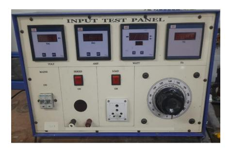
Input test panel is portable easy to use for finding all four parameters to approve the quality of any type of electrical appliances or device with digital display of voltage, current, wattage as well as frequency at desired ac voltage and load.
