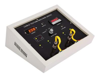
Mobile charging/DATA /AUX and many other cables can be test or compare with help of this instrument, this test cable sequence and shorting after it gets ok it inject real current up to 5 amp and with help of voltage drop it provides the capacity of cable with digital current meter, a 6 digit counter also provided to count the OK production of the day, although fail indication does not fet counted.
