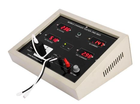
Mobile charger tester is used to test the circuit of mobile charger for production with variable electronic load up to 5Amp to ensure the quality of product. It is equipped with variable electronic load to set current at desired value with all readings like no load/on load voltage, series fail indication, input/output, voltage/current and ok/fail indication.
